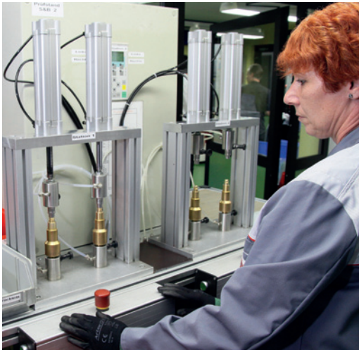
AUTOMATIC TESTING EQUIPMENT FOR GAS RETURN, LEAKAGE AND FLASHBACK TEST
